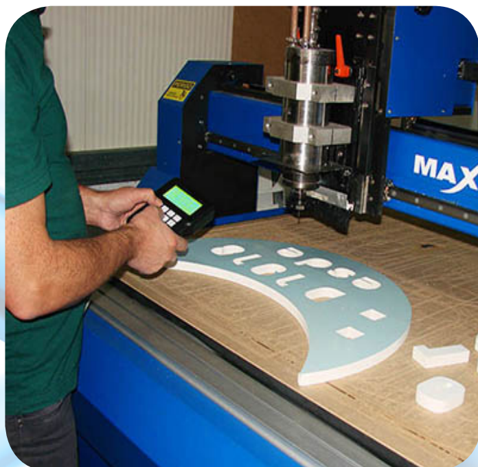
The milling cutter is able to make letters and other 3D pieces.
