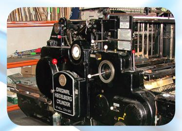
This old cylindrical **Heidelberg** was built for lead printing, but today it's used only for diecutting, taking advantage of its extreme robustness. In the back wall was there is the die-cut archive.
